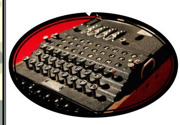
You're looking at a picture of the German Enigma Machine. This was a sophisticated device used to transmit and receive encoded messages. Nazi scientists were so confident in their creation, they considered the code to be unbreakable. Configured properly, the device could scramble secret military messages over  $1.5 \times 10^{20}$  ways. Ultra was the codename given to British efforts to
